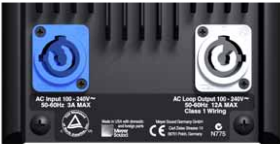
UPJunior AC Input (left) and AC Loop Output (right) Connectors
