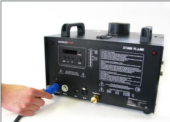
Turn off the Stage Flame power button and disconnect the powerCON cable and DMX plugs.
