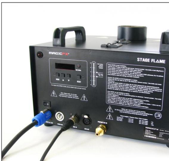
Connect the other end of the DMX cable (male plug) to a professional DMX controller.
