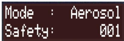
Press MENU again to save your selection. Now the DMX addresses need to be entered. First, the “safety” address needs to be set. You select the desired channel by using the UP and DOWN buttons. Press the MENU button to save the setting.
